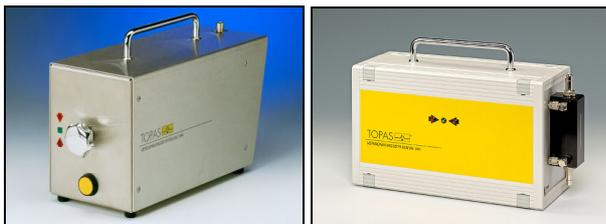
Dilution System DIL 554 and DIL 540 (automatic readjustment)
